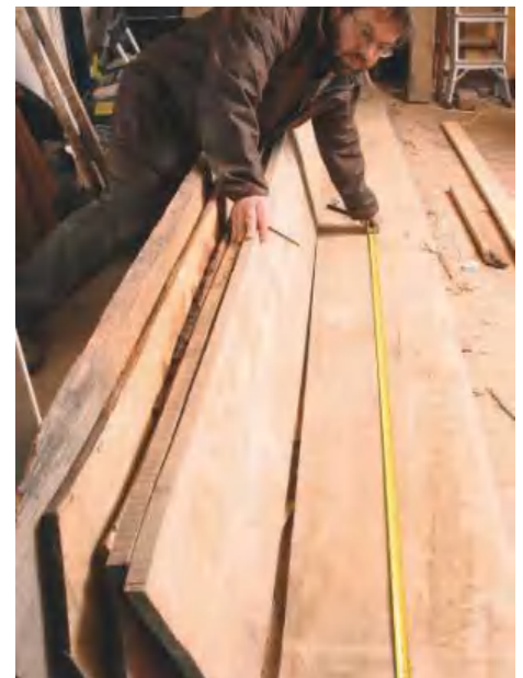
▲ Pic.13 Once you have found the right material of the right quality, you need to measure out the boards
